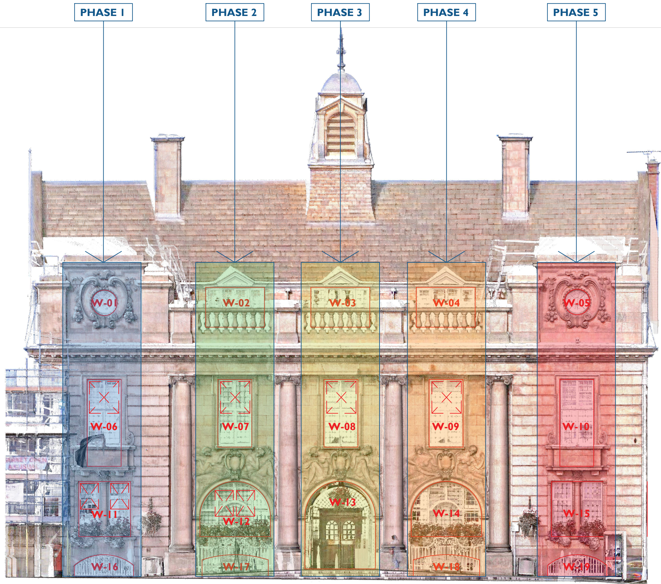
2 PHASING WITH INDICATIVE SCAFFOLDING ZONING 2010 1:100 @ A1 X TEMPORARY GLAZING (PERSPEX) LOCATION
